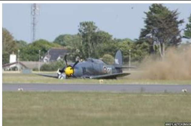
Unlocked right undercarriage asymmetric yawing moment on landing caused aircraft to slew off runway. (Photo: Ron Weldon)
