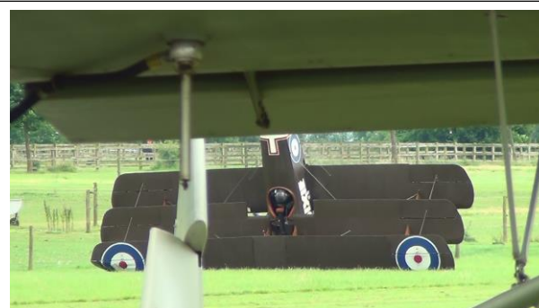
Interaction between left wheel and fence post during final approach saw the Triplane flip onto its nose on landing. (Photos Aviation Safety Network)
