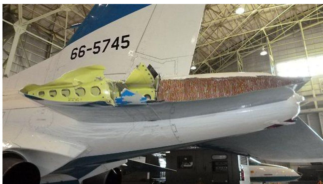
#2 Managed to retain control of the aircraft and land with only one segment of the horizontal tail plane intact. (Source AFP)
