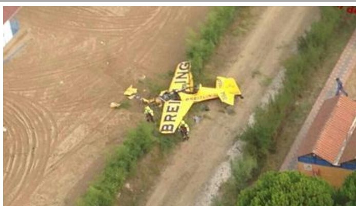
The near horizontal attitude at impact kept the aircraft intact; fortunately, no post impact fire. (Photo: www.documentingreality.com )
