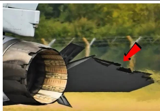
The delaminated composite on the right hand stabilator caused the pilot to terminate the display and land asap. (FLYHIGH.NEWS, Elwyn R)
