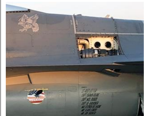
The F-16 pulls vapor as the missing panel is visible. (Photo: Tom Demerly/-TheAviationist.com)
