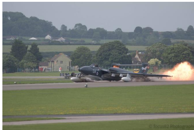
With no other option after hydraulic failure, a wheels-up landing was the only other alternative for the Sea Vixen. (Scott Dabinett)
