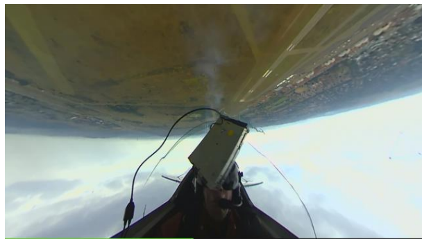
The VHF radio flies out of the instrument panel, narrowly missing Hopkin's face and impacts and cracks the canopy. (Nigel Hopkins)
