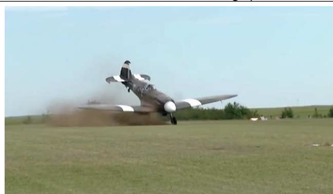
Early rotation during take-off enabled the propeller to dig into the soft runway when engine torque depressed the right oleo. (Service Communication Mairie de Lounguyon)
