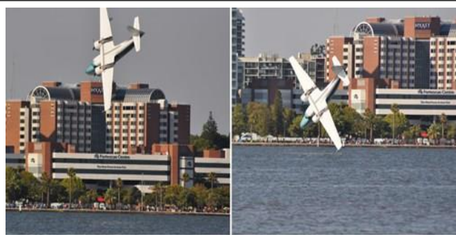
Consistent with an aerodynamic stall, the bank angle increased and the nose pitched down as the Mallard impacted the Swan River. (Mike Graham)
