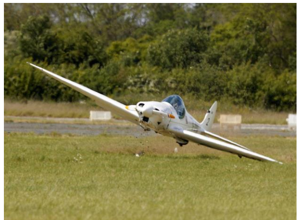
With very little excess energy available for a 'flared landing' or undercarriage extension, the Twister 'pancaked' on-field. ( https://www.youtube.com/watch?v=Y3hARxTtCtI )
