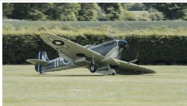
Seafire high angle of attack, hard landing impact of left wheel flipper door and wing tip. (Airplane Pictures, Nigel Paine)
