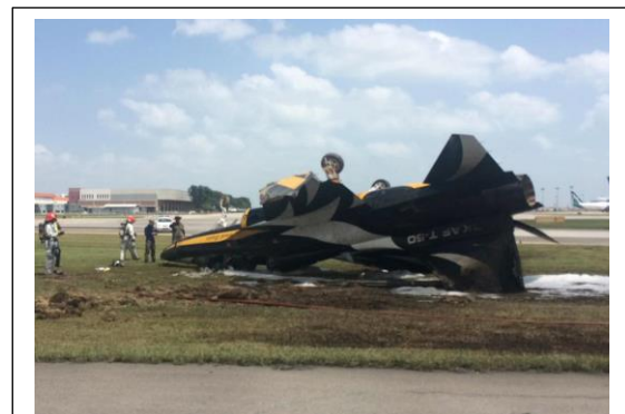
ROKAF Golden Eagles T-50 rolled over on departing the runway after bursting a tyre during a formation takeoff. (TODAY)
