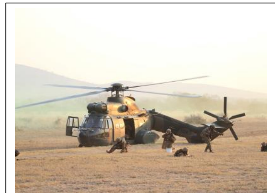
Could the enthusiasm of providing an impressive 'quick stop' to the mainly military spectators have resulted in the chopper entering vortex ring state?
