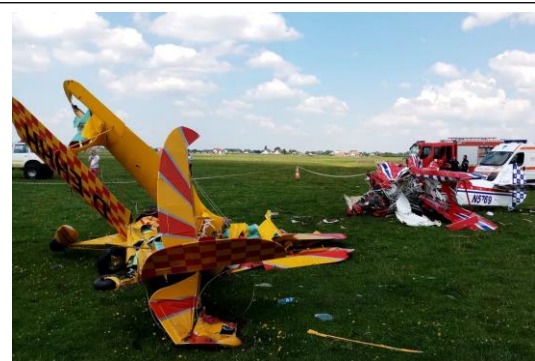
Without sufficient longitudinal separation, the wingman rolled into Lead during the mirror roll to erect. (Romania, Graphic Animation)
