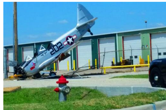
Fuel starvation resulted in engine failure of the PT-23. (Jason Tidd)
