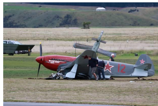
The Yak 3 right hand wing was torn off when it clipped a cherry picker at Warbirds Over Wanaka . (Liam Parker)
